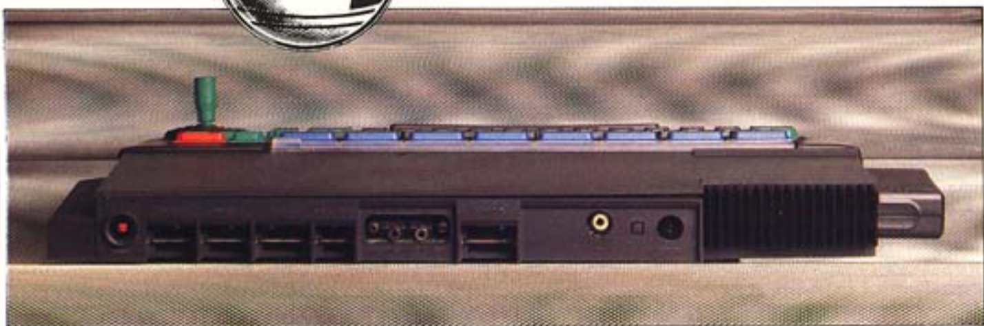
From left to right: reset switch, joystick, serial and parallel ports, cassette sockets, monitor and UHF output, powersocket
