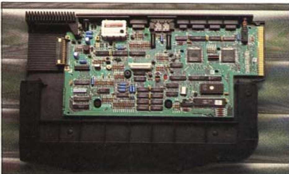
A compact PCB with the two custom chips overshadowing the Z80 processor
