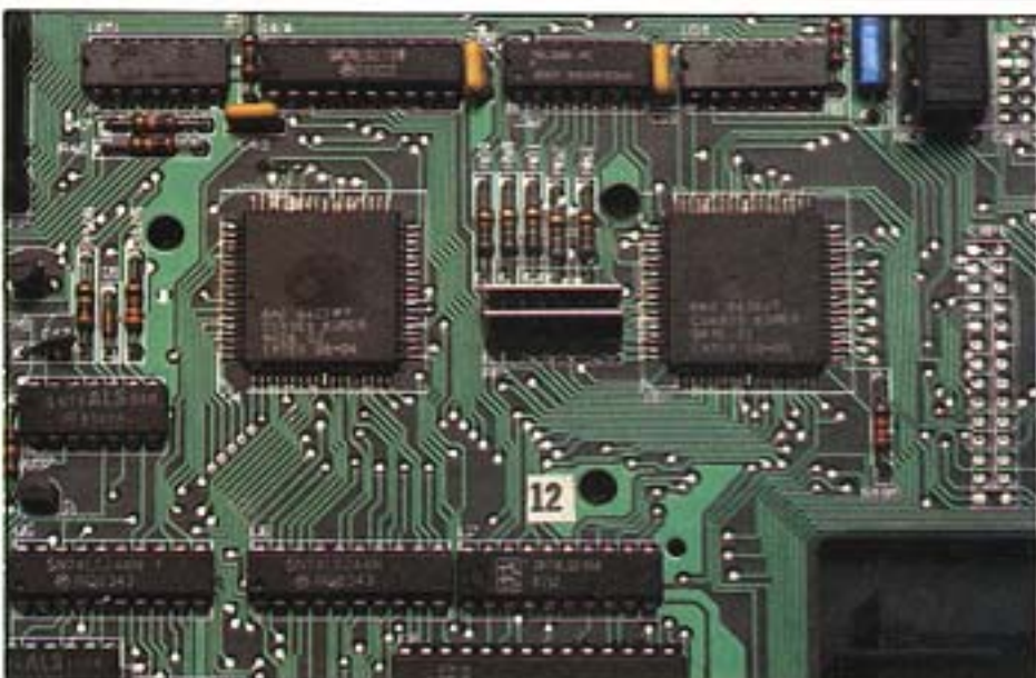
The custom video and audio chips, 'Nick' and 'Dave' — named after the designers
