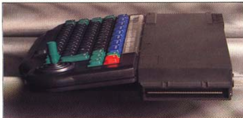
The expansion port with no fewer than 62 lines for peripheral connection
